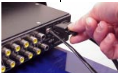
connect cable to "DATA IN," and terminator to "DATA OUT"
